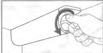
2. The cartridge will eject slightly with a clicking sound.
